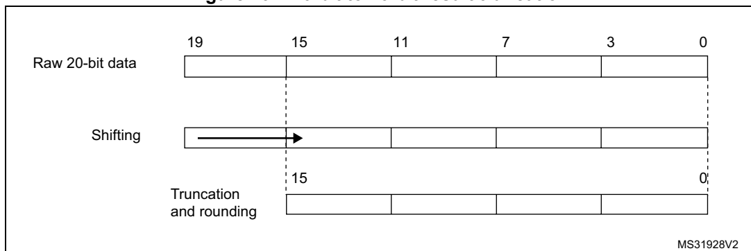
Figure 297. 20-bit to 16-bit result truncation
